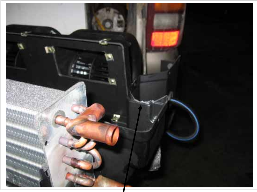
Plastic cut out of this area for evaporator fitting.
