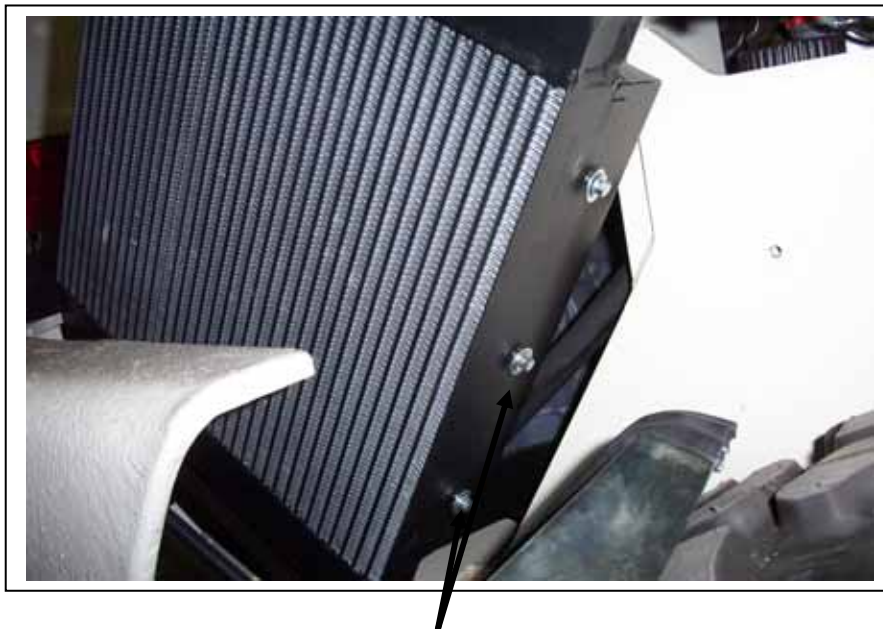
Large OD washers installed on existing bolts
