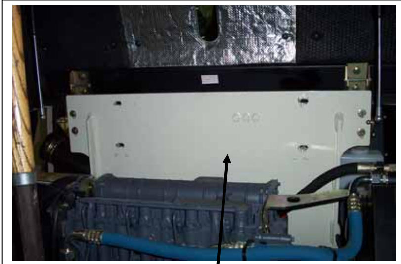
Muffler and exhaust pipe removed
