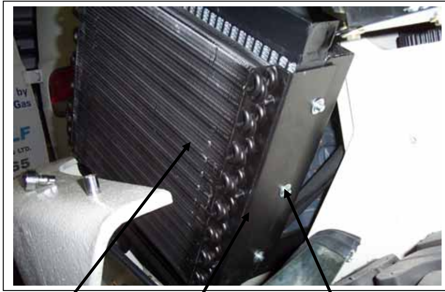
Condenser coil Condenser bracket M8 bolts
